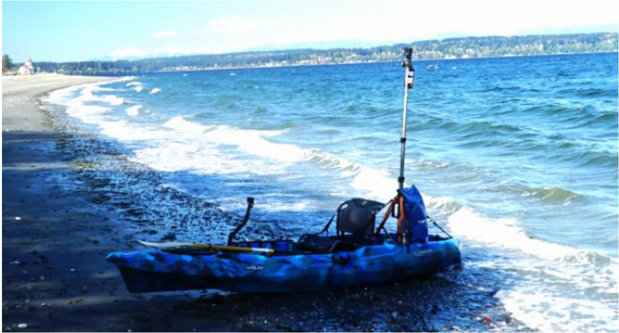
Figure 1. Kayak surveying platform. Tripod camera mount on stern.
