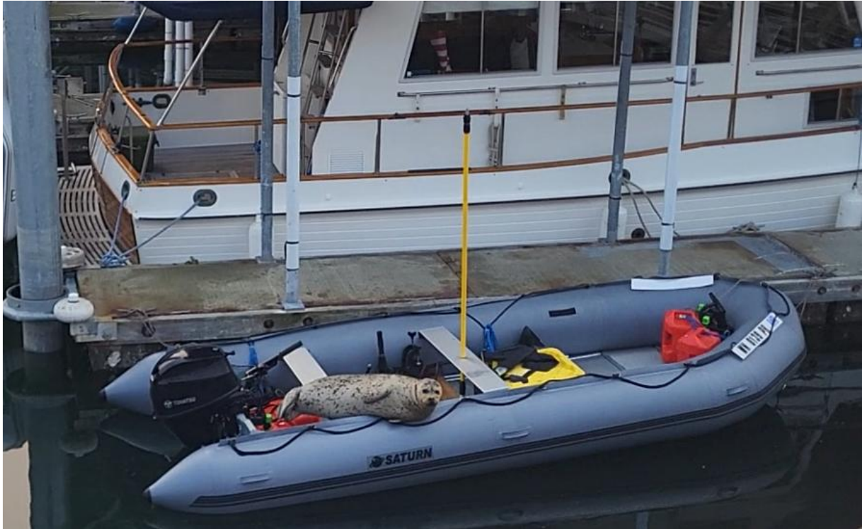
Figure 2. Eighteen-foot inflatable with guest. Yellow mast for camera mount.
